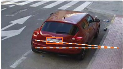
Too small (less than 130px wide) Tilt angle exceeds 5°
