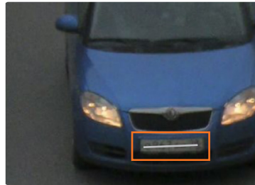
Improper focus settings. Adjust the lens.
